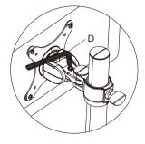
To adjust the screen angles use the 5x5 allen key supplied
