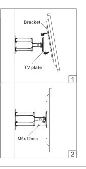
Tighten or loosen the M6 screws on the TV plate to keep it level
