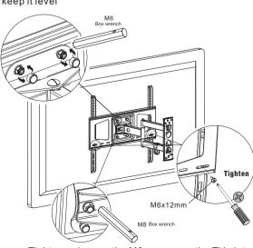
Tighten or loosen the M8 screws on the TV plate to adjust the tilting function
