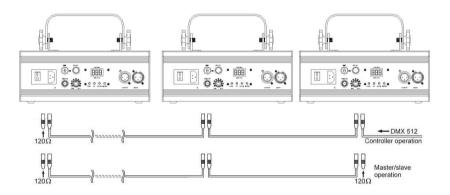
**Caution:** At the last fixture, the DMX-cable has to end with a terminator. Solder a 120 Ohm resistor between PIN 2 (-) and PIN 3 (+) into a 3-pin XLR-plug and plug it in the DMX-output of the last fixture.
