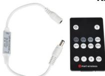
In-line controller for low voltage 12-24Vdc single colour LED tape with DC jack input and output. Controlled via the supplied handheld RF 14-key remote control with access to dimming and built-in pattern programs for dynamic displays and mood lighting applications.
