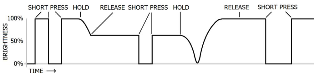
Using the above method, the ILD2 enables full switching and dimming control from a single press switch, which can be any wall mount or in-line momentary switch.
