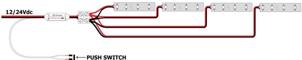
Beyond the maximum length of tape (8A current), it will be necessary to use single colour LED amplifier/repeaters (153.770UK, 153.771UK) to extend dimming control to additional lengths.
