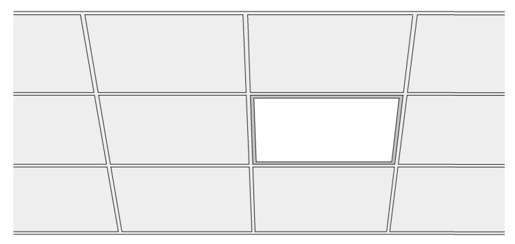
If there is no ceiling grid, a panel may be hung from the ceiling using the suspension kit supplied. The kit comprises 4 steel cables, 4 flanged ceiling anchors with screws and 4 M10 fasteners. This kit enables suspension of the LED panel for up to 1m from the ceiling.
