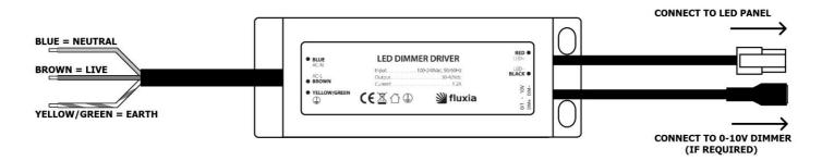
The output side of the LED driver has 2 wires. One is an EL power lead which connects with its counterpart on the LED panel and the other is a male DC5521 jack socket which can receive 0-10Vdc control voltage for PWM dimming. When the DC5521 jack is not connected, the LED driver operates as normal at full output to the LED panel. If a standard 0-10Vdc dimmer is connected to the DC5521 jack, the LED panel will operate as a dimmable luminaire.
