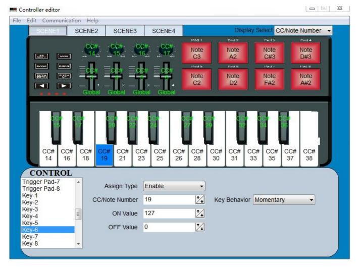
The twenty-five keys of the keyboard will function as independent buttons to transmit control change messages. You can specify which MIDI channel the control change message is transmitted on, whether or not each key is enabled, the key type, the control change number, as well as the On and Off value.
