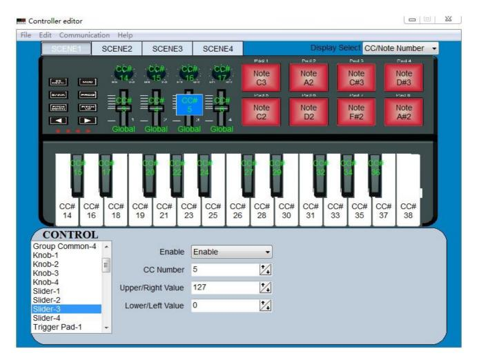
Operating a slider will transmit a control change message. You can enable/disable each slider, specify its control change number, and specify the values transmitted when the slider is moved fully upward or fully downward.
