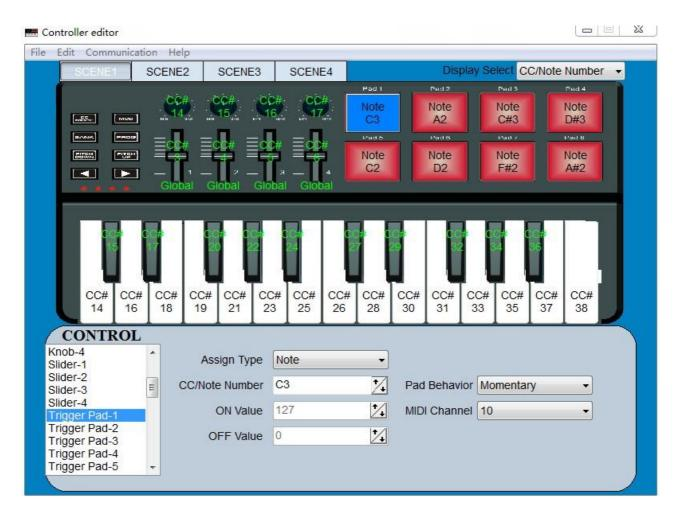
Depending on the assign type, the trigger pads can transmit note messages or control change messages. For each trigger pad, you can individually specify the assigned message, the MIDI transmit channel, the behavior of the trigger pad, the note number, the control change number and the values transmitted when the pad turns on or off.
