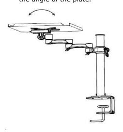
**2.** Attach your selected sized plate to the arm of the bracket and secure with the plastic stopper and screw
