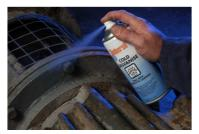
Cold Galvanising Spray is a unique combination of zinc powders and resins, formulated to form a high performance zinc-rich coating that actively fights rust and corrosion by its galvanic properties. Ferrous metals are protected by the sacrificial action, even when scratched or damaged. Zinc becomes the anode which is attacked by corrosion and the base metal the cathode. A film of water-insoluble zinc oxide is formed, which stops rust and corrosion.
