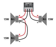
Ensure that the combined impedance connected to each speaker output is not lower than  $4\Omega$  and that the speakers connected can handle the output power at that combined load impedance.
