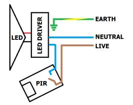
Connection to the PIR and LED driver are concealed within the rear weatherproof housing.
